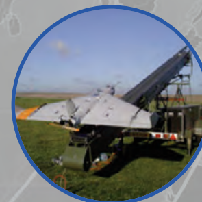
X-48B Boeing Research & Technology Mass and inertially scaled, 8.5%, subscale demonstrator 6.4m wingspan 80 test flights so far
