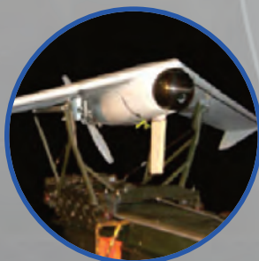
Min0 1.4m span, 11kgs Fully autonomous point & click operation. Gust-insensitive advanced control
