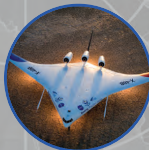
X-48B Boeing Research & Technology Mass and inertially scaled, 8.5%, subscale demonstrator 6.4m wingspan 80 test flights so far
